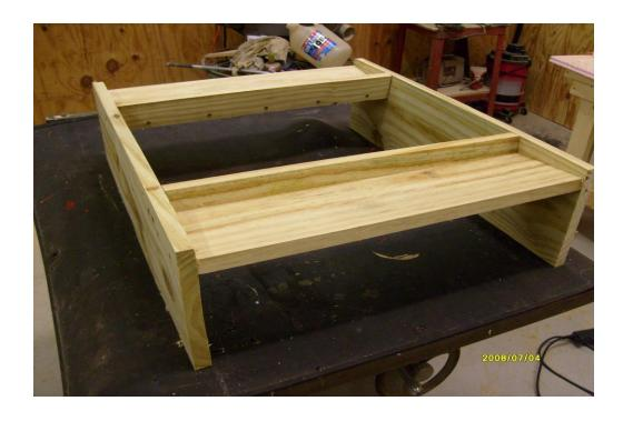
Temporarily clamp Side Rails and Top Brace as shown. Side Rail should be flush with top of Top Brace.
